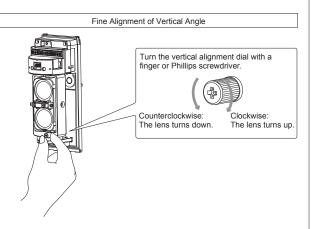
3 Adjust the horizontal and vertical angles while checking the light receiving status by Alarm indicator LED on the pairing receiver.
