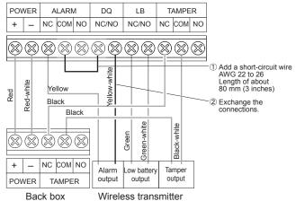
Wiring example when Using N.C. Transmitters b) Canceling the alarm output in adverse weather conditions
