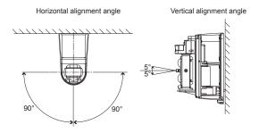
Optical alignment is an important adjustment to increase reliability. Be sure to take adjustment steps 1 through 5 described below to attain the maximum level of the output through the monitor jack.
