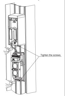
After completing the settings and operation check, insert the tamper bushing into each transmitter/receiver.
