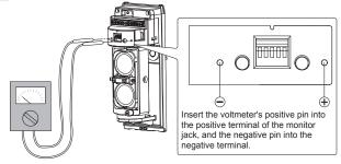
5 Set the voltmeter range to 5 to 10 VDC.
