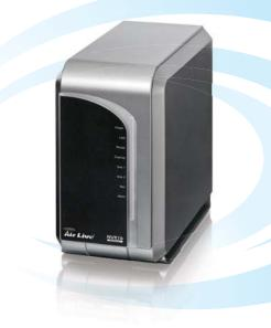
hard drivers and raises its capacity up to 2TB; with the H.264 video compression format, it could keep video clips for more than 200 hours (4Mb bitrates per channel).
